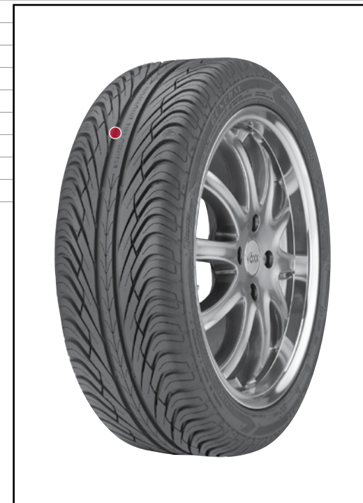
• Dot shows location to make tread depth remaining measurement.
